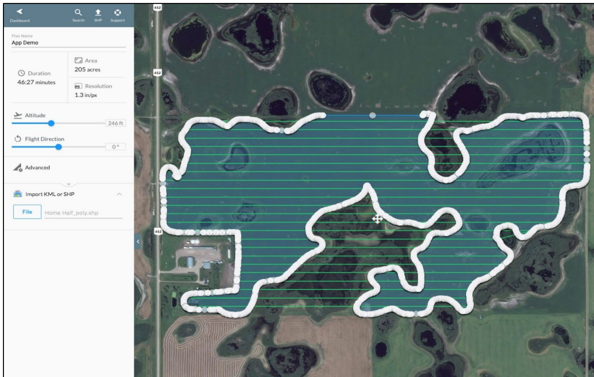
Figure A3.2. Flight plan interface example using the Drone Deploy app (Taken from Waltham 2020).
