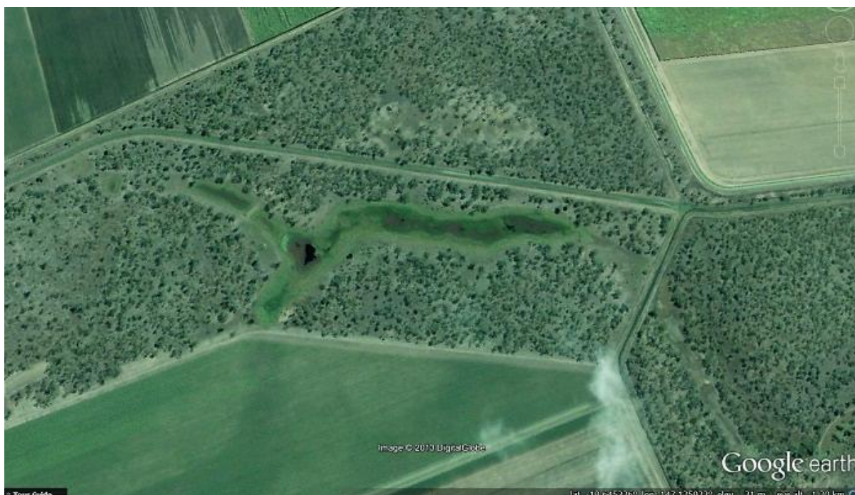
Figure 15. Circumventing of floodplain palustrine wetlands by constructed drainage networks. Palustrine wetlands on the Barratta Creek floodplain circumvented by areal drainage networks at Green Swamp1 West Barratta Ck catchment.
