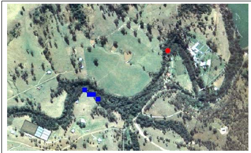
Plate 1. Riverine Wetlands from the Tweed area that are not mapped as a water body. Water bodies (blue) were mostly obscured by vegetation or were too narrow for satellite pixels. Accuracy assessment sample point shown by red dot.
